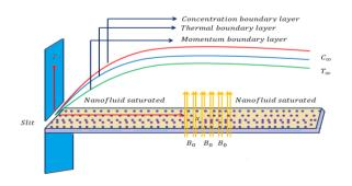
Fig. 1: Schematic flow diagram.
