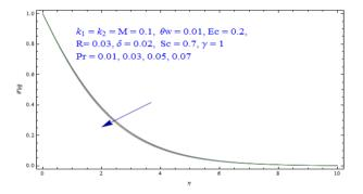
Fig. 7: Influence of Pr on temperature distribution.
