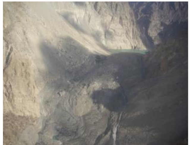
Figure 3: A NE aerial view of the Attabad landslide Source: FOCUS Pakistan, it triggered from the left side and blocked the narrow gorge of Hunza River and KKH. The debris material traveled 800m upstream and 1200m downstream while the length of the actual blockage was almost 950m. Totally the spread of the landslide debris was approximately 3km. The downstream surges damaged 8 houses in which 19 deaths occurred. Lacustrine deposits clay and silt
