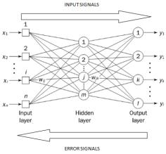
Fig. 8. Multilayer neural network structure
