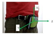
Fig. 3. Placement of the IMU and processor board
