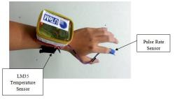
Fig. 4. Prototype of the vital-sign monitoring device
