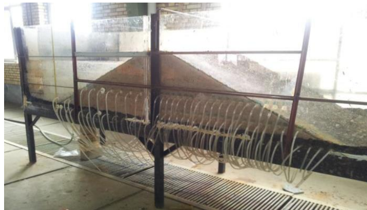
Figure 2. The experimental model of the earth dam and the piezometers mounted in the body of the model (bottom-up photograph)
