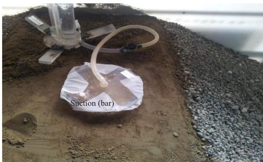
Figure 5. Suction system for disk installed on the body of the dam to measure unsaturated hydraulic conductivity
