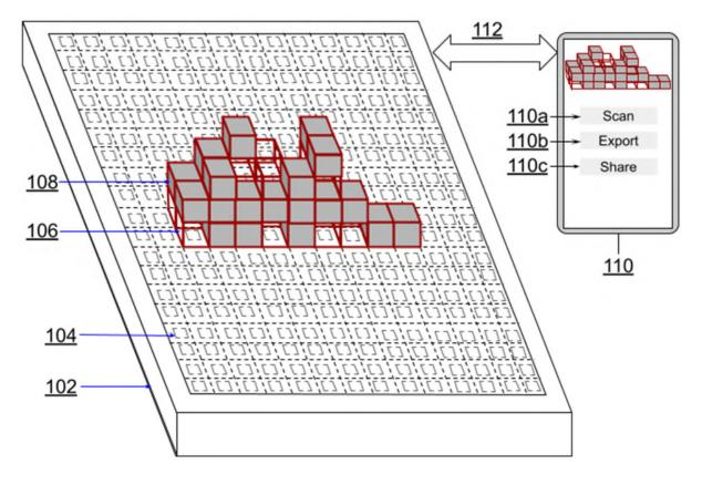
Fig. 1: A hardware interface and accompanying software to intuitively model voxel-based 3D objects
