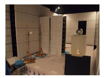
(c) Fig. 3.20. Scenario of experiment in a radio anechoic chamber: (a) Experimental layout, (b) measurement scenario, and (c) usage of microwave absorber to suppressed direct wave.
