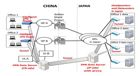
Fig. 2: Our cloud-based system provided in China
