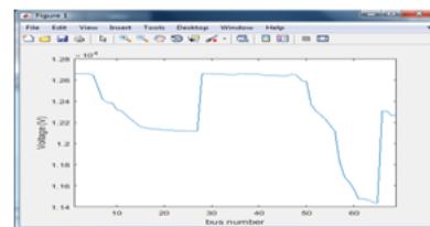
Fig 4.7 Voltage profile 69 Node system after reconfiguration
