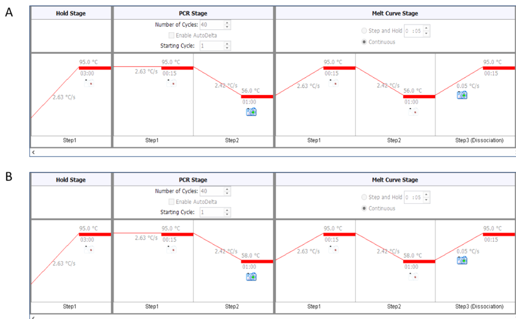
Figure 2. Details of the PCR setup. Detailed information of the PCR setup on the ViiA7 instrument with telomere primers (A; annealing at 56 °C) and human \beta -globin primers (B; annealing at 58 °C) is provided. Cycling temperatures with time, number of cycles, as well as ramping rates are clearly indicated here. A melt curve analysis is added at the end of 40 cycles of PCR to ensure the absence of primer-dimers.
