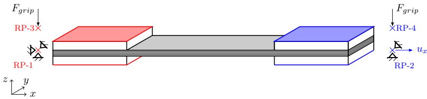
Figure 3.28: Tabbed coupon model applied on simulations. Red and blue faces represent the tied to the reference points, corresponding in colour, where displacement BCs and gripping loads are applied. Representation adapted from [193].
