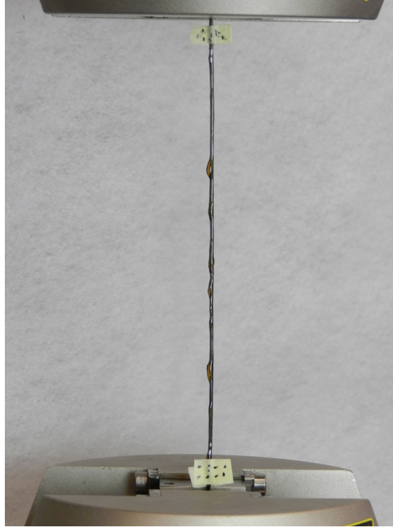
Figure 3.3: Shear member tow sample in test machine.
