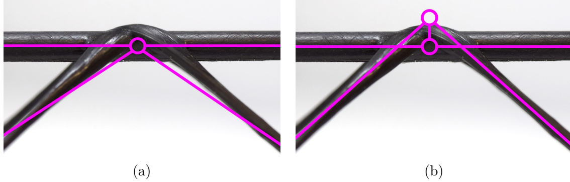
Figure 4.1: Joint geometric idealisation methods: a) Concentric; b) Eccentric.
