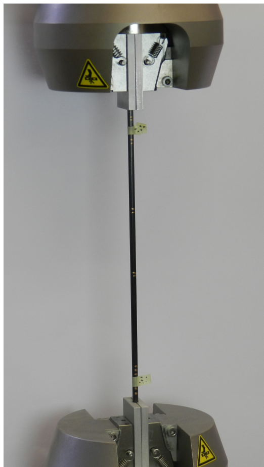
Figure 3.1: Tensile testing of chord member pultrusion tubes.
