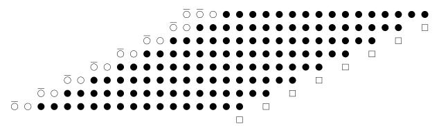
Fig. 3.3. Partial product matrix of the exact  $16 \times 16$  radix-4 Booth multiplier. •: a partial product. O: a sign-extension term.  $\overline{O}$ : an inverted sign-extension term.  $\square$ : a sign-correction term.
