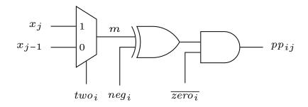
Fig. 3.2. Gate-level schematic for exact PPG.
