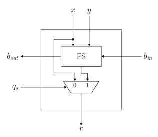
Fig. 4.1. Circuit-level schematic for EXRDC.
