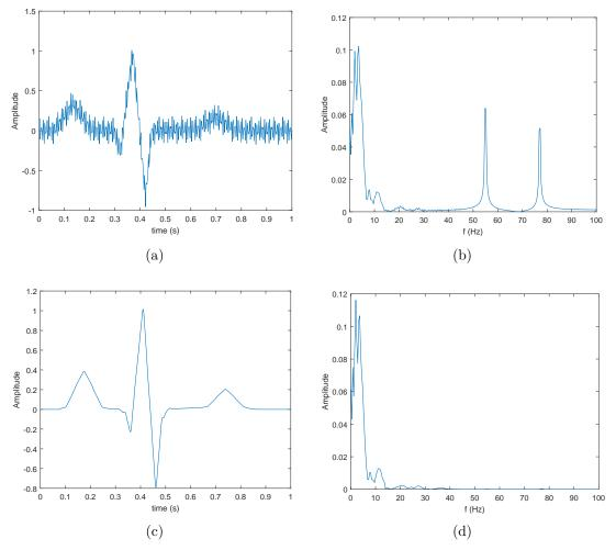
Fig. 3.11. Input electrocardiograph signal in the (a) time domain and (b) frequency domain. Signal outputted by the low-pass FIR filter in the (a) time domain and (b) frequency domain.
