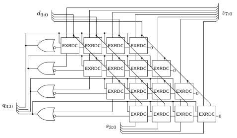
Fig. 4.2. Architecture of exact 8/4 restoring divider.
