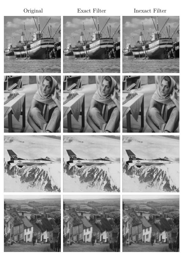
Fig. 5.9. Images used in  $7 \times 7$  Gaussian blur application from top to bottom: boat, barbara, airplane, and goldhill. The first column contains original images used as input, the second column is the result from convolution computed using exact operations, and the third column contains the outputs of the convolution computed by ABM-MAC.
