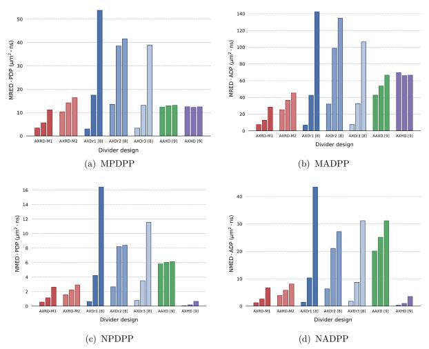
Fig. 4.7. Graphs illustrating accuracy-hardware tradeoff metrics for the implemented dividers.
