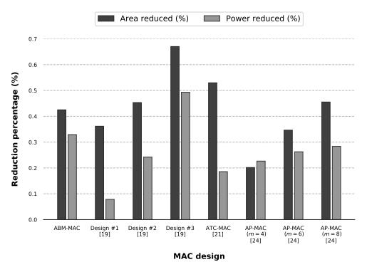
Fig. 5.3. Hardware savings for approximate MAC units compared to the accurate design.
