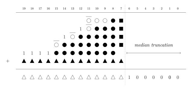
Fig. 5.1. Bit matrix of ABM-MAC in which the partial product bits generated by the multiplication are summed along with the accumulator value in a single computation. The k = 6 least-significant bits of the result are truncated to the median value.  $\bullet$ : exact partial products,  $\bigcirc$ : sign-extension terms,  $\blacktriangle$ : inexact partial products,  $\blacksquare$ : accumulator bits from the prior computation,  $\square$ : newly-computed accumulator value.
