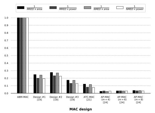
Fig. 5.5. Inverse multiplication of error metrics (MRED and NMED) by hardware parameters (area and power) to evaluate tradeoff.
