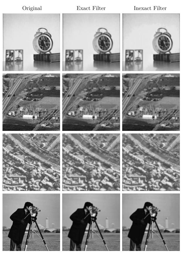
Fig. 5.7. Images used in  $5 \times 5$  Gaussian blur application from top to bottom: clock, chemical plant, aerial, and cameraman. The first column contains original images used as input, the second column is the result from convolution computed using exact operations, and the third column contains the outputs of the convolution computed by ABM-MAC.
