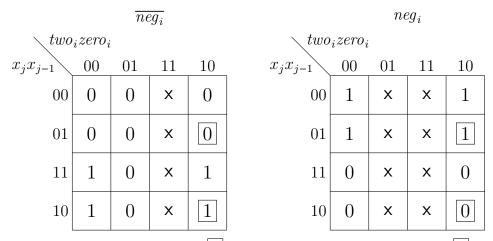
Fig. 3.4. Karnaugh-map for PPG-2S, where 1 represents a change from 0 to 1 and 0 represents a change from 1 to 0.
