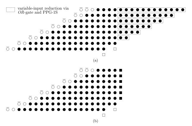
Fig. 3.9. Partial product matrix of ABM-M3 for k = 12, where (a) indicates the row-wise groups over which  $x_j$  is reduced, and (b) shows the reduced matrix.  $\bullet$ : an exact partial product.  $\blacksquare$ : an inexact partial product generated by PPG-1S.  $\circ$ : a sign-extension term.  $\overline{\circ}$ : an inverted sign-extension term.  $\Box$ : a sign-correction term.
