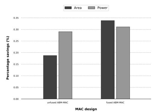
Fig. 5.4. Comparison of hardware savings delivered by fused vs. non-fused ABM-MAC.
