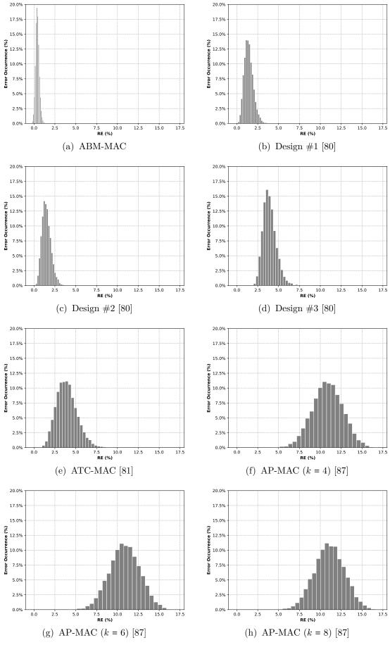
Fig. 5.2. Relative error distribution for implemented MAC units.
