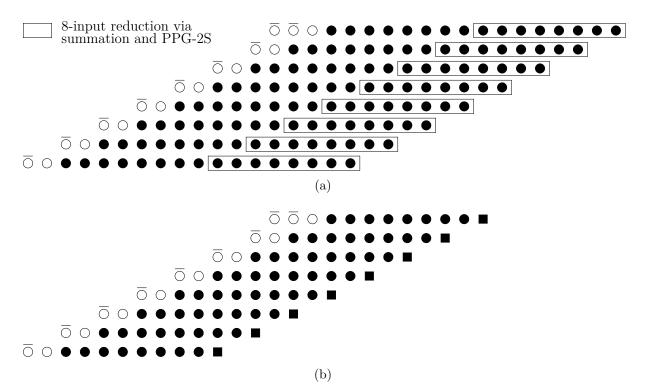
Fig. 3.7. Partial product matrix of ABM-M2 for k = 8, where (a) indicates the row-wise groups over which  $x_j$  is summed, and (b) shows the reduced matrix.  $\bullet$ : an exact partial product.  $\blacksquare$ : an inexact partial product generated by PPG-2S. O: a sign-extension term.  $\overline{O}$ : an inverted sign-extension term.
