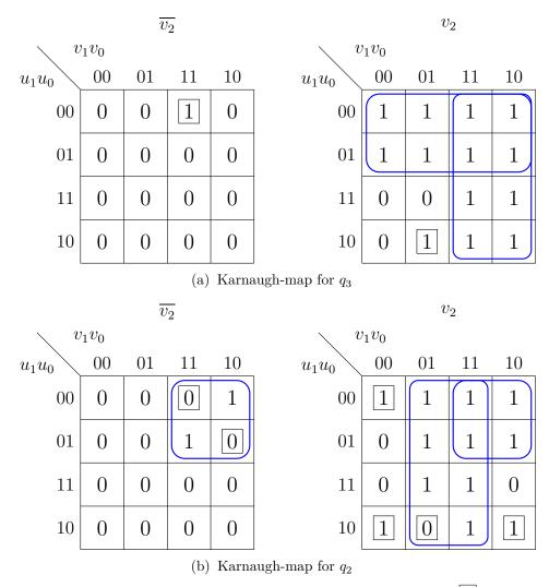
Fig. 4.6. Karnaugh-map for further approximating  $q_3$  and  $q_2$  in AXRD-M2, where 1 represents a change from 0 to 1, 0 represents a change from 1 to 0, and a blue box indicates approximated terms.
