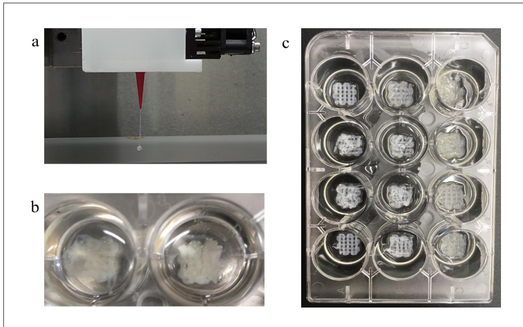
Figure 3-6 Difficulties during the 3D printing procedure of EW-1.5% Alg blend. Unattached strands leading to clogging the needle (a), instability of the printed structure in the crosslinker bath (b), and low fidelity and resolution in printing multi-layer construct
