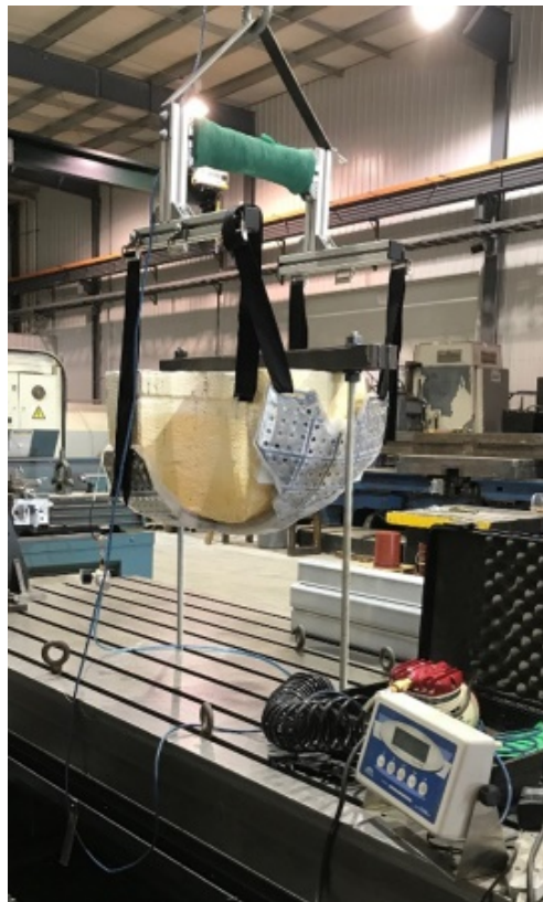
Figure 3.15. Strength testing set up for the prototype IIb breastplate. The breastplate was loaded with 227 kg, which was verified by the load cell attached above the H-frame on the breastplate.
