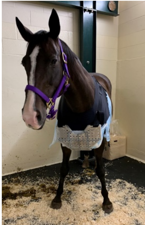
Figure 3.11. Horse spreading front legs due to the pressure caused by Prototype IIa. The horse stood with a broad base in an attempt to reduce pressure on the insides of the legs.
