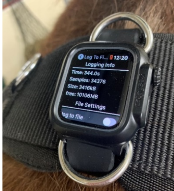
Figure 4.2. Apple Watch IMU used in the experiment.
