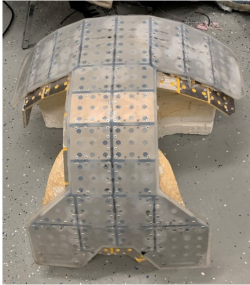
Figure 3.8. Second prototype breastplate (Prototype IIa) made of steel plates connected via seatbelt webbing. The seatbelt webbing ran through the steel plates and was riveted together. Holes were drilled in the metal plates to allow for greater bonding of silicone.
