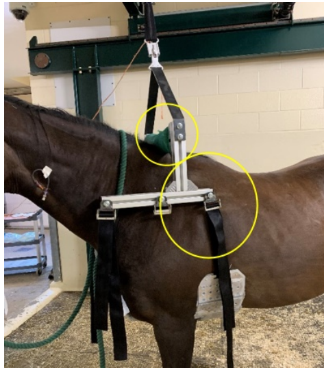
Figure 3.17. The Prototype IIb and H-frame on the horse used for weight compensation trial day 1. The yellow circles highlight the areas that required modification. The bar running across the top of the horse required an extension to pull the breastplate straps out and up to try and reduce pressure “squeezing” inwards on the abdomen.
