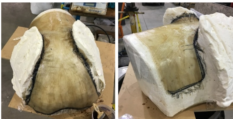
Figure A.9. The negative mould was used to shape the fibreglass shell made from two layers of fibreglass cloth and fibreglass resin.
