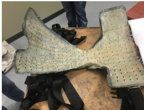
Figure A.26. Image of the air hoses through the fibreglass that were inserted into each air pocket.
