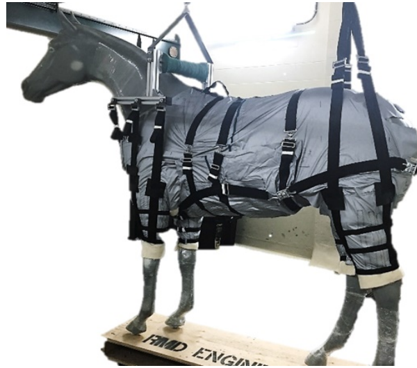
Figure 3.3. EARL, the model horse, used for initial safety testing and fitting of the rehabilitation harness prototypes (example displayed above, harness prototype and H-frame used in previous studies) and breastplate.
