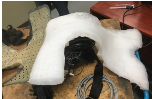
Figure A.25. Removal of silicone air pockets in an attempt to re-bond and seal air pockets. Silicone separated from fibreglass during initial testing.
