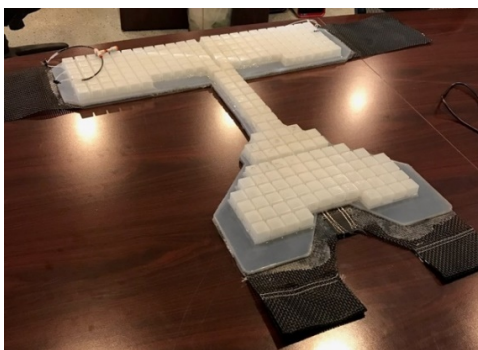
Figure 3.19. The breastplate silicone was removed from the previous support material (steel plates), and fibreglass webbing was incorporated for support. The fibreglass webbing was placed in a silicone mould in the shape of the breastplate. Silicone was poured and cured to encase the webbing. Silicone air pockets were attached to the silicone encasing the webbing.
