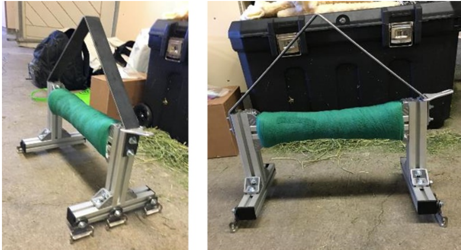
Figure 3.2. The H-frame used with the harness prototype to remove inward pressure on the shoulders and direct the straps outward.
