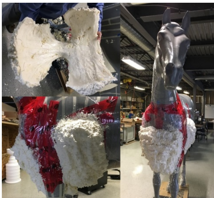
Figure A.8. The breastplate was created from a spray foam mould of EARL, the Styrofoam model horse used for testing. We began by covering EARL in saran wrap and spray foaming on top to create a mould of EARL's chest. From the mould, we created a negative mould with spray foam, mimicking EARL's shape to create a fibreglass shell.
