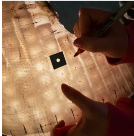
Figure A.13. A light was shone through the silicone to mark the holes in the bottom of the air pockets. A small metal disk was used to line up with the air pocket, and a permanent marker was used to mark each hole.
