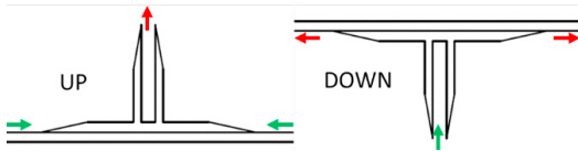
Fig. 4. Infusion set-ups 'Up' (left) and 'Down' (right) with arrows representing direction of resin flow.
