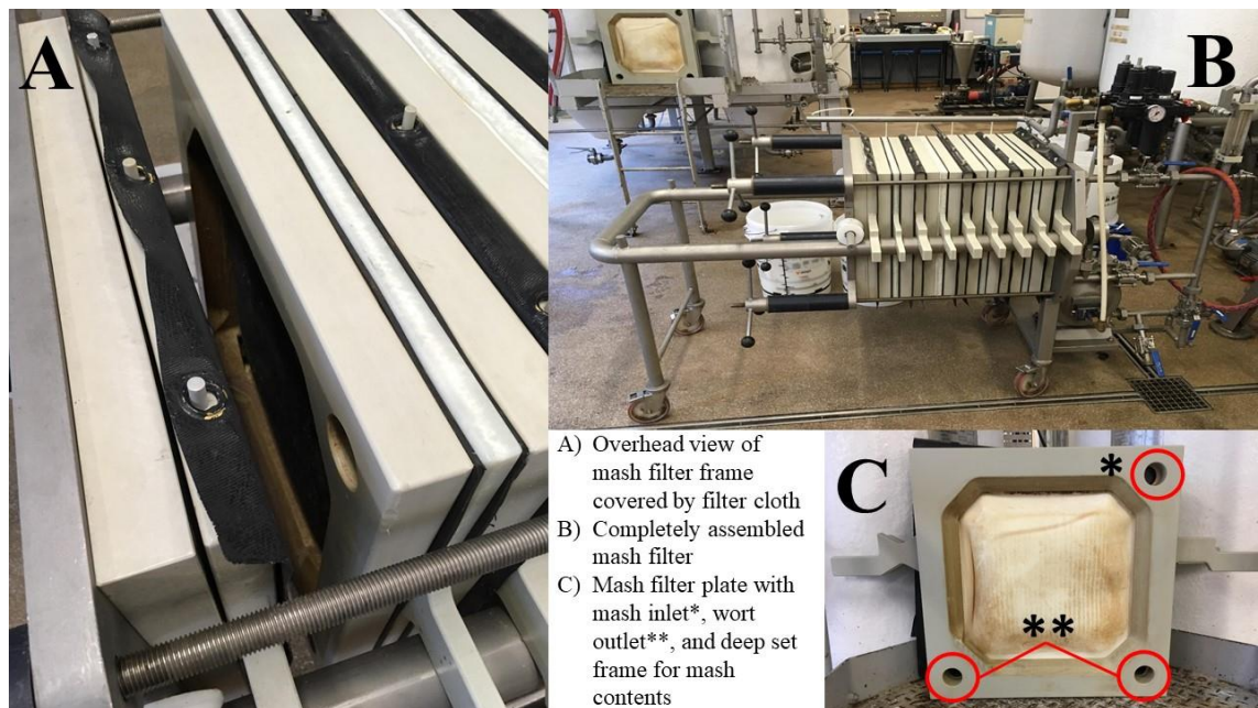
Figure 1.2- Mash filter and mash filter components- A) Overhead view of mash filter frame covered by filter cloth, B) completely assembled mash filter, C) mash filter plate with mash inlet(indicated by one red circle and a *), wort outlet(indicated by two red circles and **), and deep set frame for mash contents to flow into.
