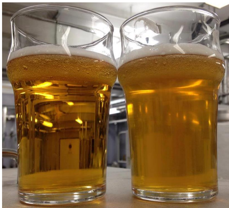
Figure 1.11- Demonstration of sporadically turbid samples (right) compared to samples within specifications (left), source-industry partner.
