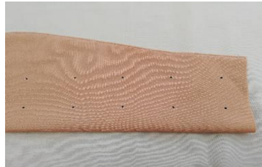
Figure 12. Pressure garment with measurement lines marked with dots for placement of sensors
