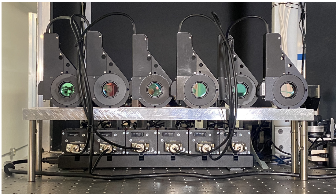
Figure 2. The new polarimetric hardware installed on the MIRC-X optical bench at CHARA. The top panel shows the half-wave plate assembly ① and motor control boxes ② in relation to the MIRC-X instrument during initial testing in 2019 November, where calibration was conducted with a pair of linear polarizers ③. Not pictured is the mini-PC, which is installed above the MIRC-X table, controlling the motor boxes via USB. The bottom panel shows the waveplates “beam-on” during on-sky observations in 2020 November.
