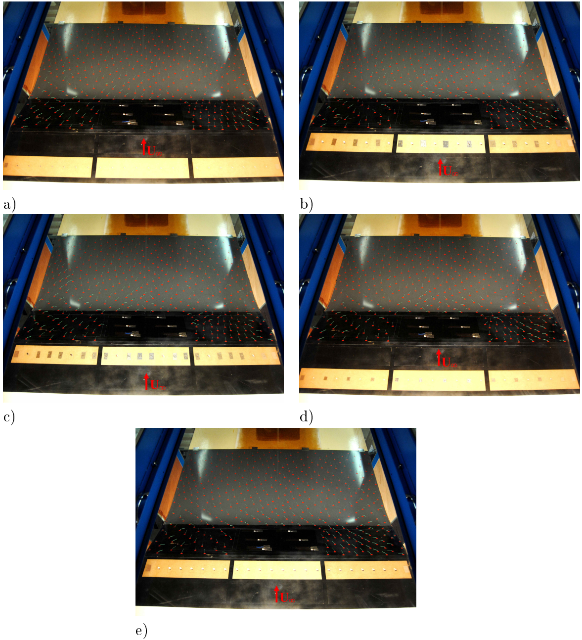
Figure 5.2: Wool tufts visualisation for a) FA (case 17), b) PA (case 6), c) VPA (case 4), d) S (case 20), e) FA (JD) (case 5).
