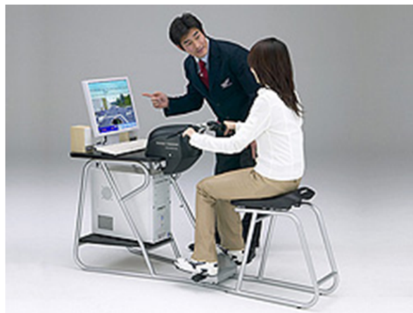
FIGURE 3.10 – Simulateur Honda Riding Trainer (Source : http://world.honda.com/news/2006/c060130RidingTrainer/ )
