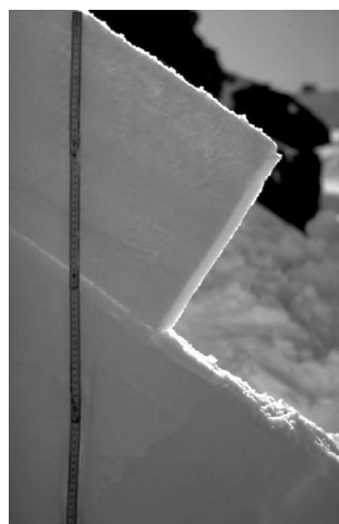
Figure 1.2: Thin weak layer of surface hoar crystals underlying a cohesive slab. From Schweizer et al. (2003).
