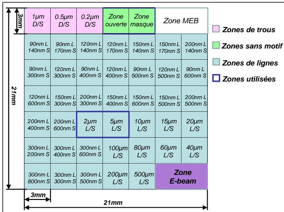
Figure 2.17: Description du masque XPS (utilisant  $\lambda=193nm$ )
