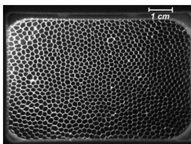
Fig. 3 Top view of a typical bubble monolayer, held in the cell schematically illustrated in Fig. 2. The osmotic pressure is 540 Pa.
