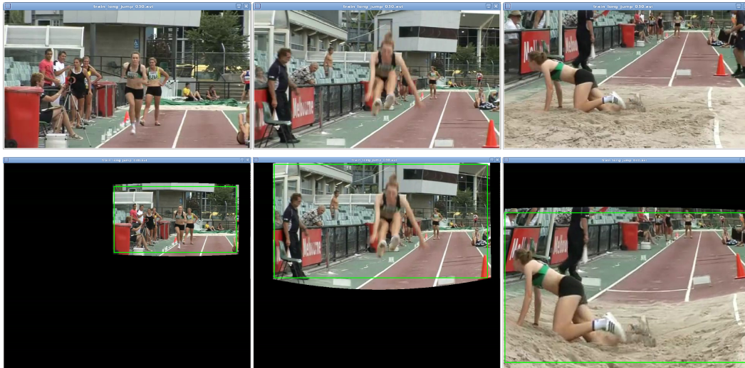
Figure 4.7: An action of the Olympic Sport [Niebles et al. 2010] dataset, before (top row) and after (bottom row) camera motion stabilization.
