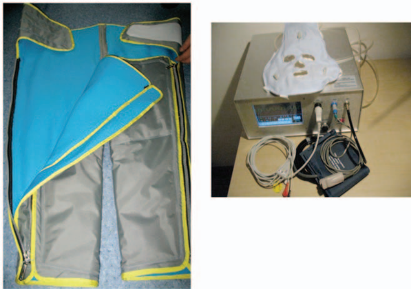
Figure 7. Pulsatile suit prototypes (human version). Left panel: pulsatile trousers. Right panel: pulsatile mask connected to a pneumatic generator and hemodynamic equipment (digital oximeter, electrocardiogram cable and sphygmomanometer cuff).
