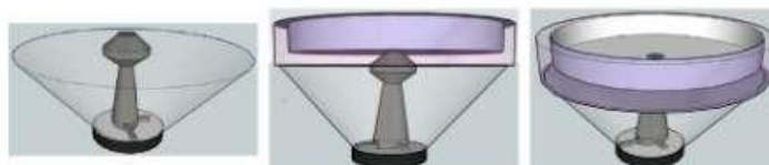
Fig. 3. Drafts showing the petri dish customization to allow the cell growth on the ATR crystal.
