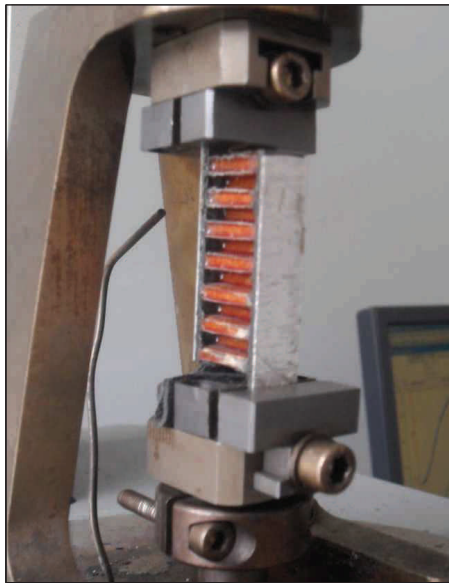
Figure 2.19: Aspect of the core shearing configuration clamped in the TMA machine
