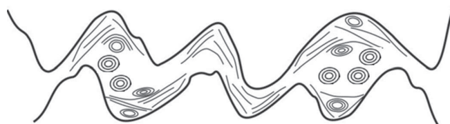
FIGURE 3.49 – Schematic presentation of nanoparticle deposition in the valleys of the surfaces which increases the real contact area. Micro-grooves (roughness valleys) act as reservoirs and help to preserve the nanoparticles within the contact. [16]
