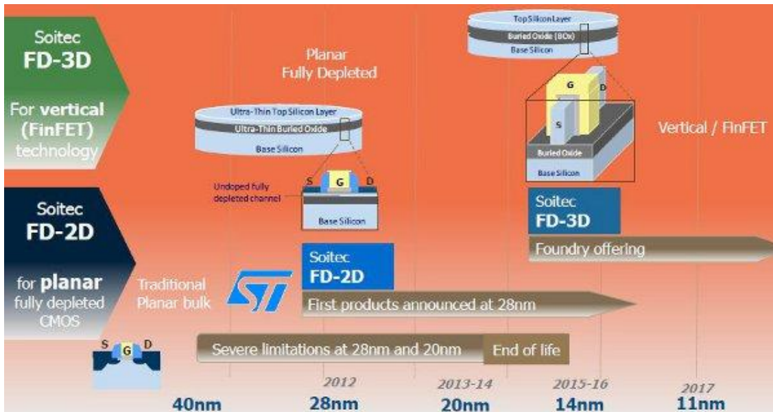
Figure I-1: SOI wafer roadmap from Soitec for next technological nodes [2].
