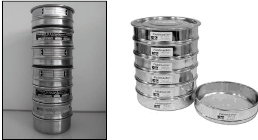
Figure 4.4: AFNOR and ASTM 3 1/2 in diameter sieves.
