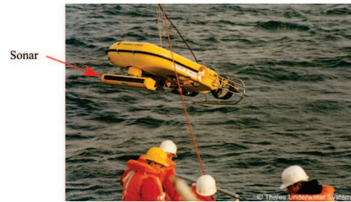
FIGURE 1.9 – PVDS de Thales Underwater Systems [36]
