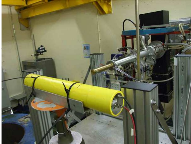
Figure 2.7: Photo of the experimental setup at the SAMES accelerator at CEA Valduc, in yellow the IC in the background the accelerator with the D/T-target.
