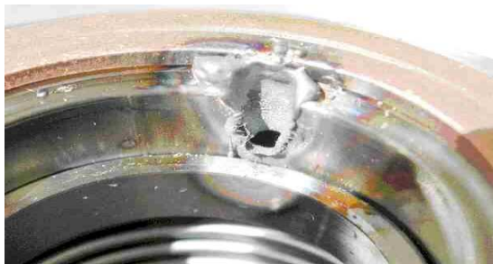
(a) Damaged inflicted to the beam pipe by the high-power electron beam of the ELBE accelerator [45].
