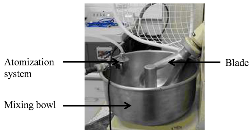
Figure III.6. Labo 25, Mahot (VMI, France) low shear mixer equipped with the atomization system.
