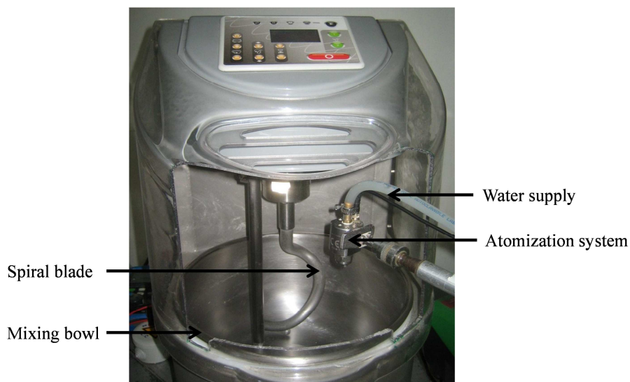
Figure III.7. Low shear mixer SPI10 (VMI, France) equipped with a spiral blade and the atomization system (Spraying Systems Co., France).
