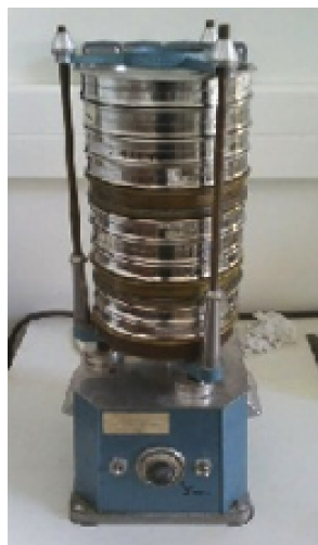
Figure III.11. Sieving device used for the size distribution measurements of wet agglomerates.
