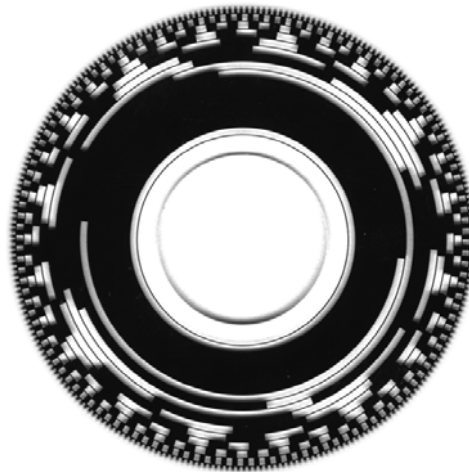
Figure 1.5 - The coded disc of the optical encoder
