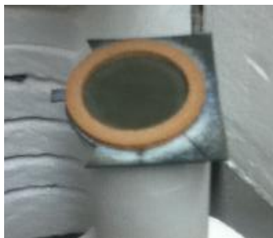
Figure IV-23: Picture of the cell BIT07 / Ni | BIT07 | GDC | PrN after ageing for 500 h at 700°C, 248 mA cm -2 (anode side).
