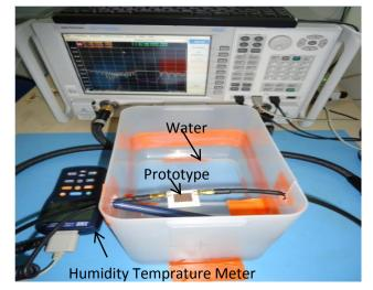
Fig.6. 4 : Measurement set-up for the sensor tag prototype.
