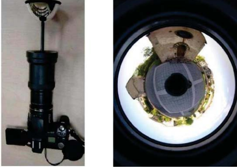
Figure 3.2: A catadioptric camera and an image taken by this camera.
