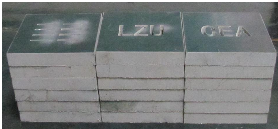
Figure 8-8. Polyethylene masks used for the neutron imaging.
