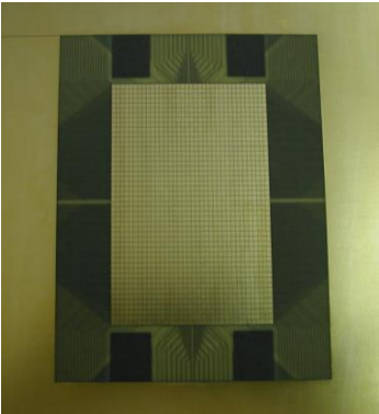
Figure 8-2. The PCB of the neutron detector (sensitive area: 57.4 mm × 88.6 mm).
