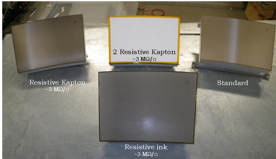
Figure 3-8. Five Micromegas modules with different anode materials.
