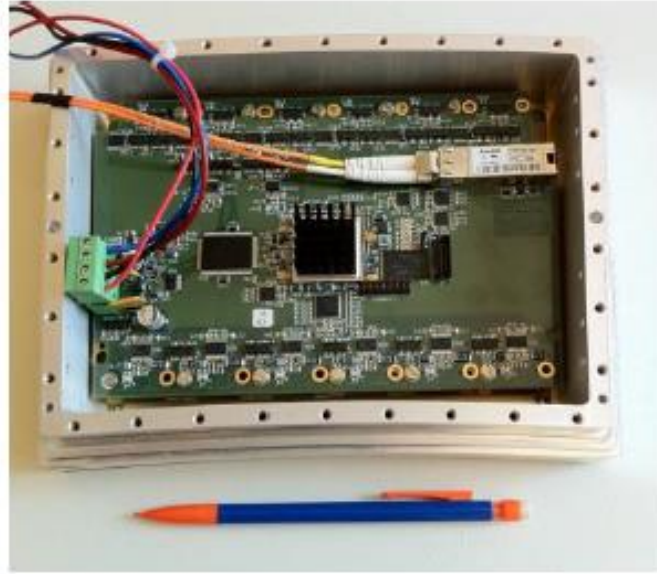
Figure 3-20. Micromegas module mounted with the new integrated electronics.
