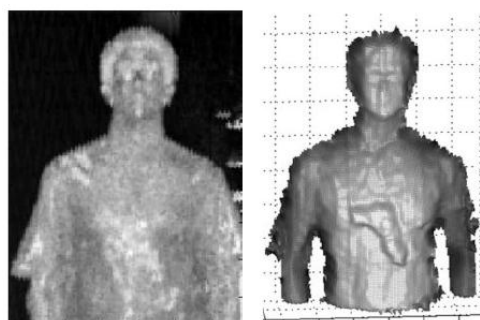
Fig. 1.10: 2D image and 3D image obtained by heterodyne detection at JPL [31]
