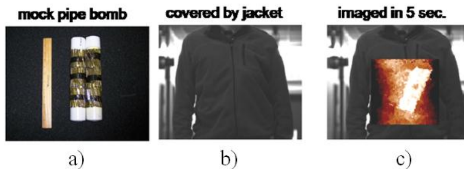
Fig. 1.11: a): Threat need to be detected; b) and c): Detection by terahertz active imaging
