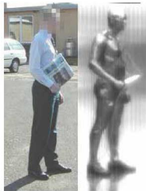
Fig. 1.8: Passive imaging at 94 GHz from QinetiQ [13]
