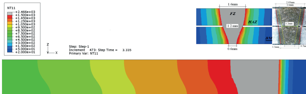
Fig.7. 8 Temperature distribution in cross section ( ^{\circ}\text{C} )
