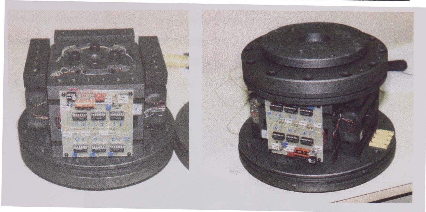
Figure C-6: Dynamometer illustrating sensing elements and gauge arrangements
