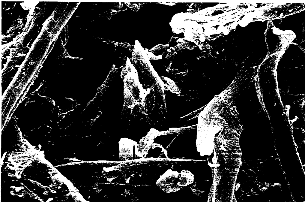
Fig. 59 SEM photograph (x500) of the 'Roma' paper fibres after laser treatment in an argon atmosphere. The gelatin size has been partially removed as a result of laser treatment.
