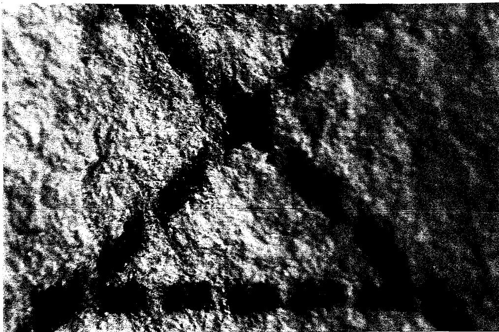
Fig. 56 Photomicrograph (x10) of the complete removal of black ball-point pen ink, from 'Roma' paper in an argon atmosphere, by a Q-switched Nd:YAG laser, using a nominal fluence of 38 \pm 11 \text{ Jcm}^{-2} .
