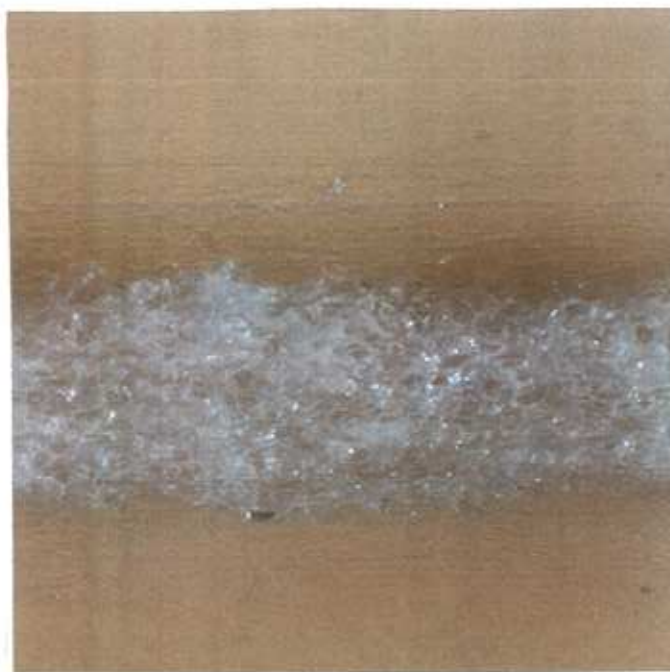
Fig. 65 Photomicrograph of the cross-section of 'Roma' cotton paper, Nd:YAG laser treated using a nominal fluence of 41 \pm 12 \text{ Jcm}^{-2} (pulse duration 87 ns), and aged for one month in a humid oven, at 90^\circ\text{C} and 50% R.H. The cross-section shows that discoloration is confined to the surface fibres only, and does not extend into the body of the paper.
