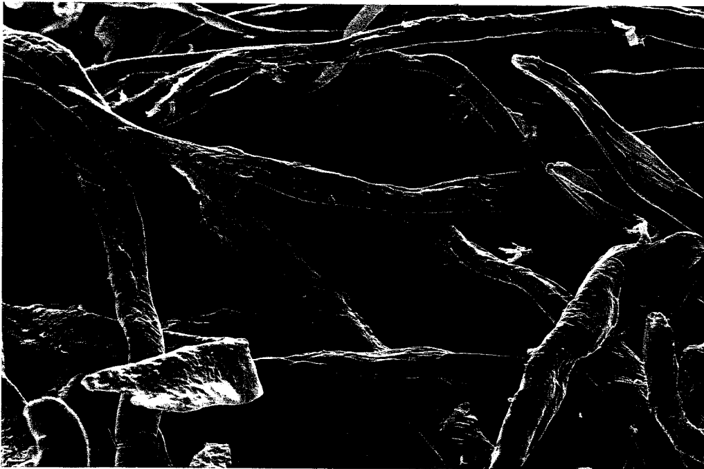
Fig. 48 SEM photograph (x400) of the 'Roma' paper fibres after laser treatment. The gelatin has been removed as a result of laser treatment.
