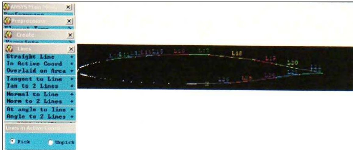
Fig. 4.5 Line connect to the created keypoints to form the profiles
