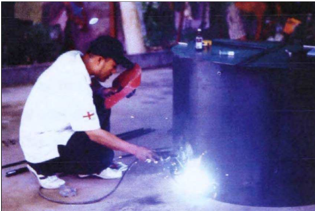
Fig. 6.40 External side welding to the end plate for S-Rotor
