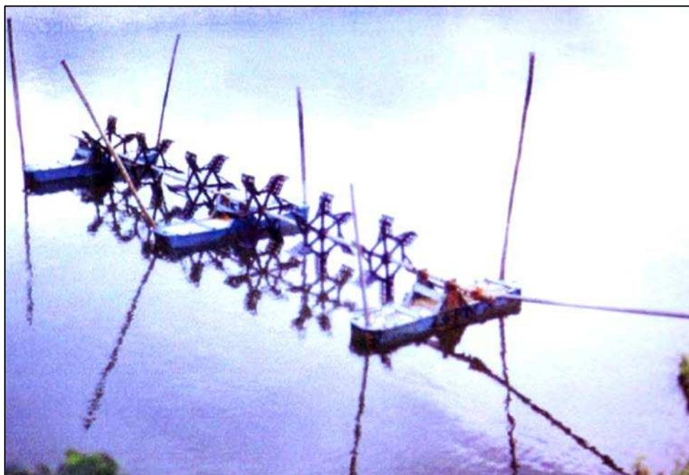
Fig. 6.38 Aerators used for the test in a shrimp farm aeration system
