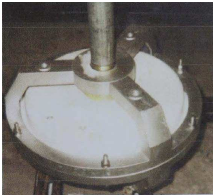
Fig. 6.8 The permanent magnet induction generator Rutland FM1803
