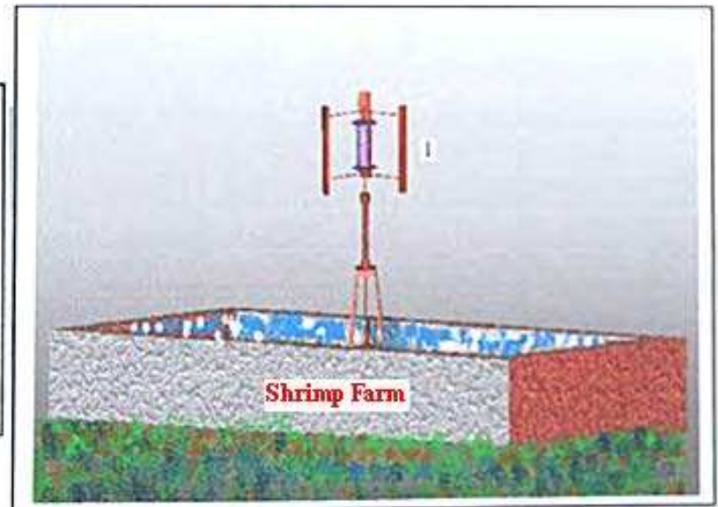
B: One unit of a wind machine for shrimp farm aeration process
