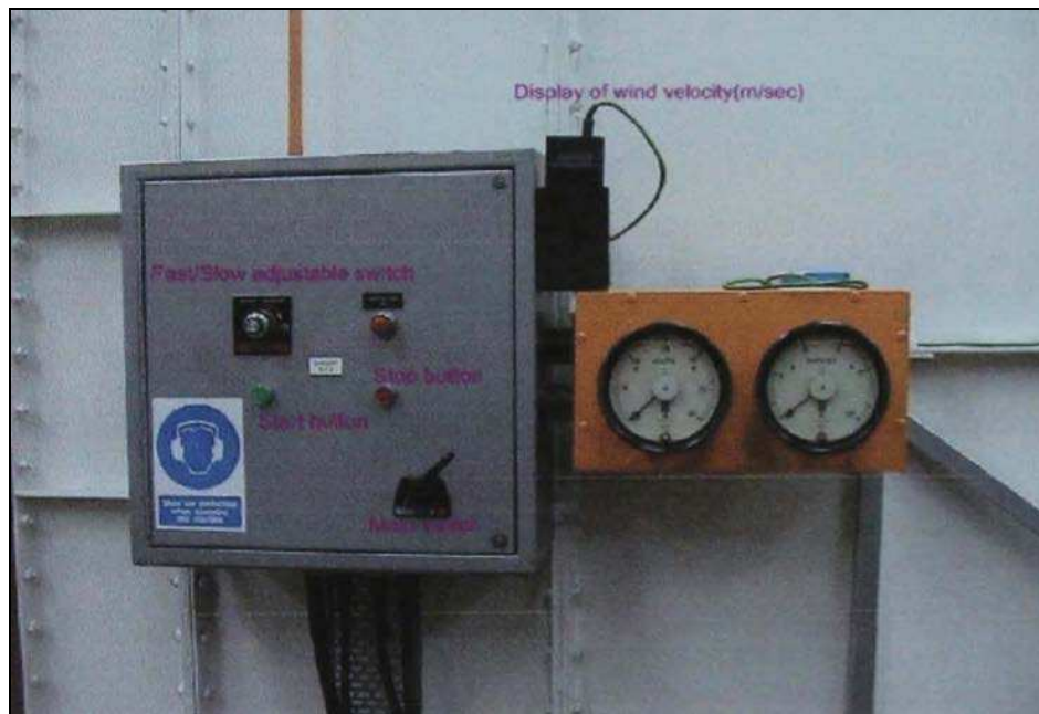
Fig. 5.9 Display and Control panel of the wind tunnel
