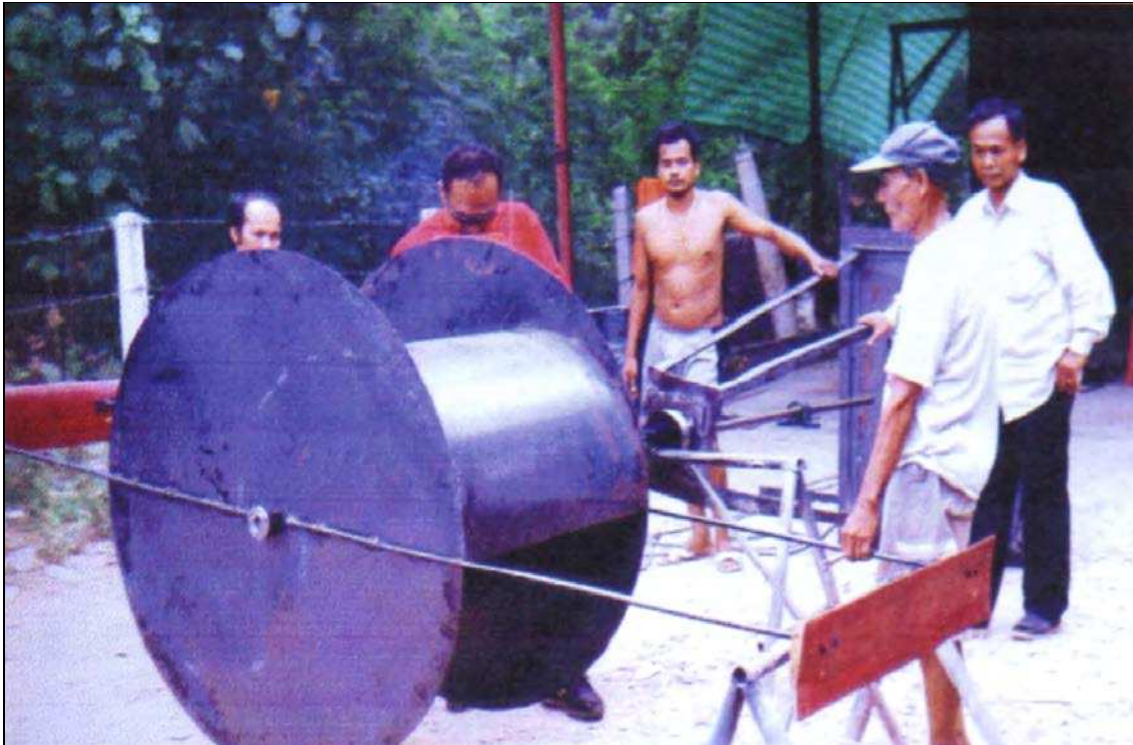
Fig. 6.41 Final welding and pre-assembling combined VAWTs
