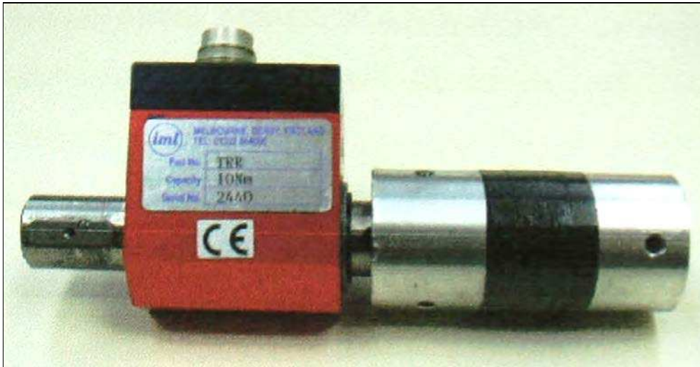
Fig. 5.11 Strain gauge torque transducer
