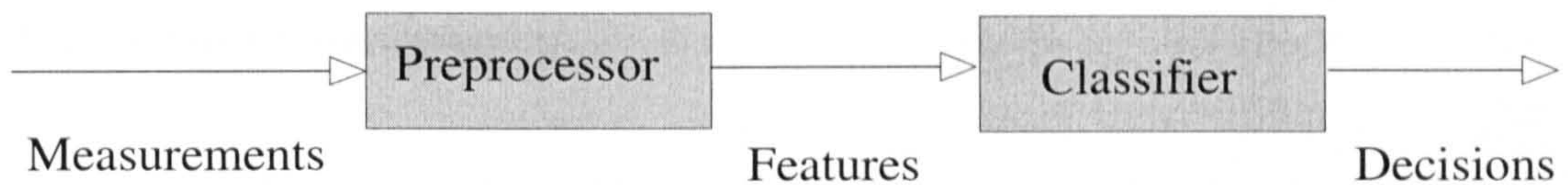
Figure 2.2 The Fault Detection and Diagnosis (FDD) process.
