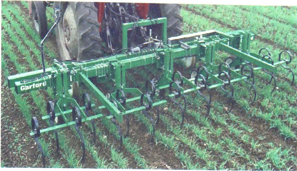
Figure 3-5 Experimental vision guided cereal hoe
