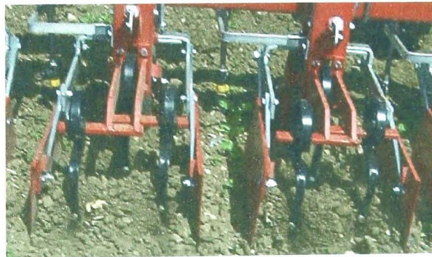
Figure 2-21 Side guards to prevent lateral soil translocation
