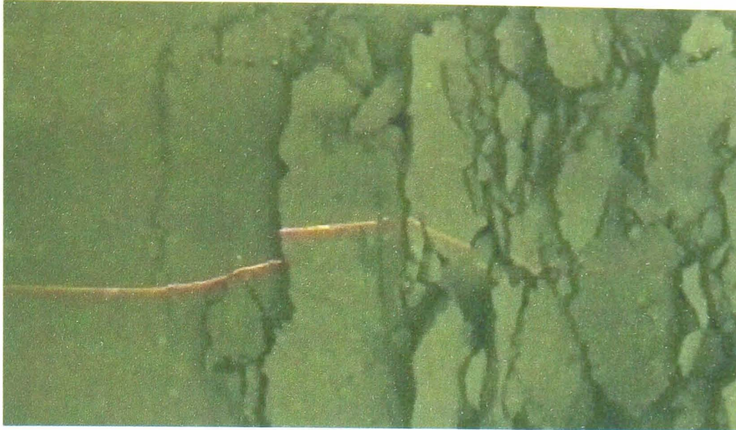
Figure 4-28 Projected laser showing in-transit height of dense soil over a 0-20 blade
