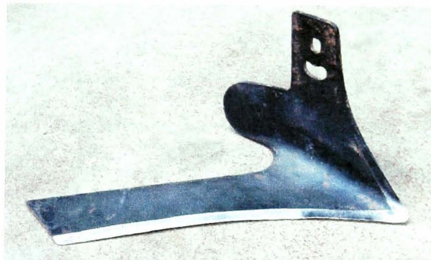
Figure 2-7 Sweep (L blade)
