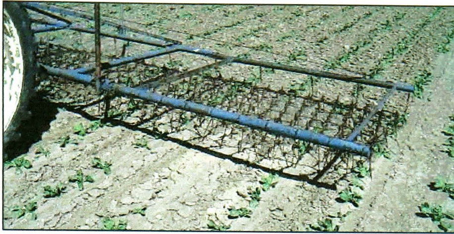
Figure 2-4 Flexible chain harrow
