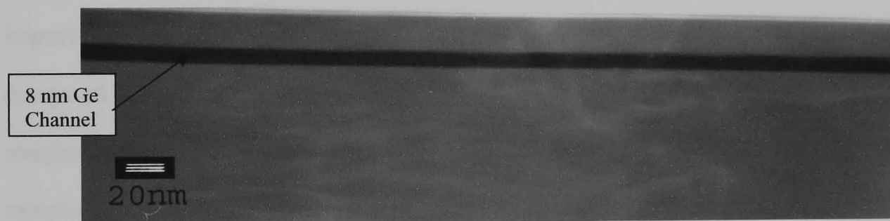
Figure 4.33. XTEM micrograph of sample 68073 showing the suppression of the upper channel roughness.
