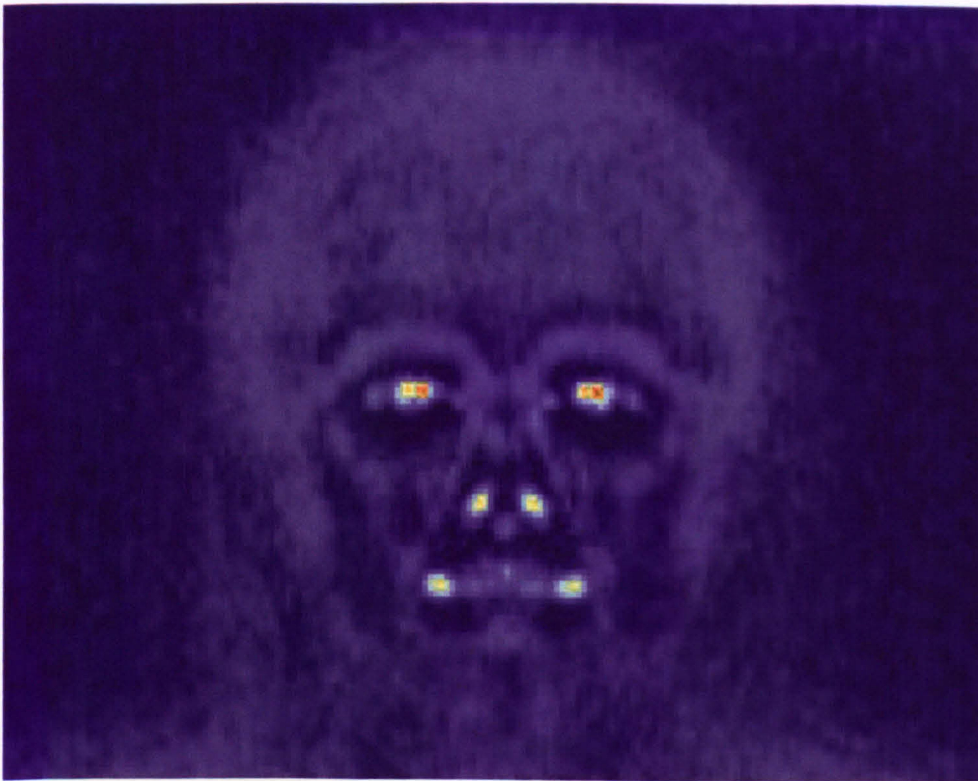
Figure 4.2: Harris corner detector success on various parts of the face, the brighter colour corresponds to higher occurrence of hits (experiment carried out by P. Bílek [BMHK])
