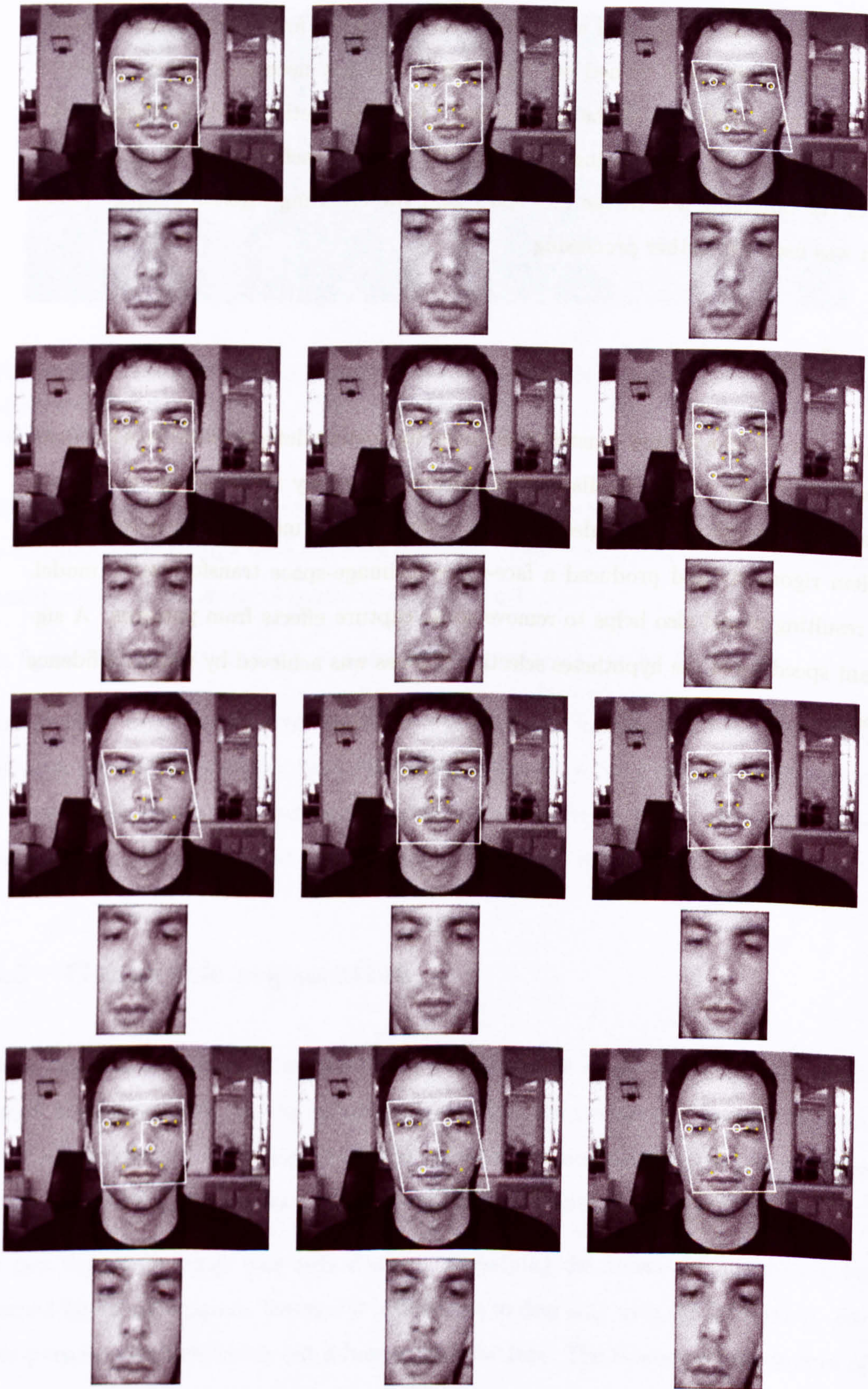
Figure 5.7: Face hypotheses 1–12 based on detected features (circled) together with the corresponding patches taken for further processing (images taken from the BioID database)
