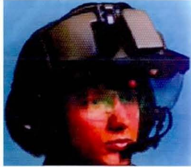
(Figure 3.7 - An optical-see-through display made by Hughes Electronics)
