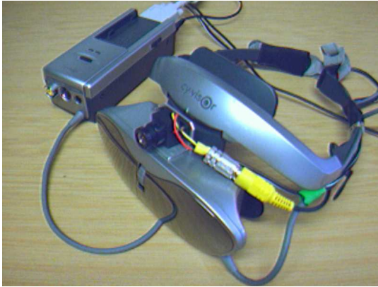
FIGURE 5.1: Cy-Visor Mobile Personal Display with mounted camera
