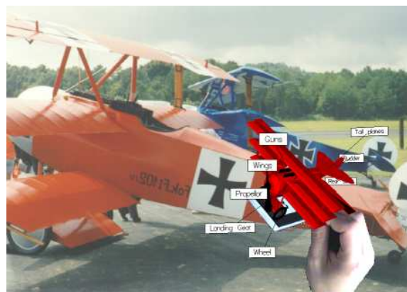
FIGURE 3.2: Virtual object and information projected onto the user's view.
