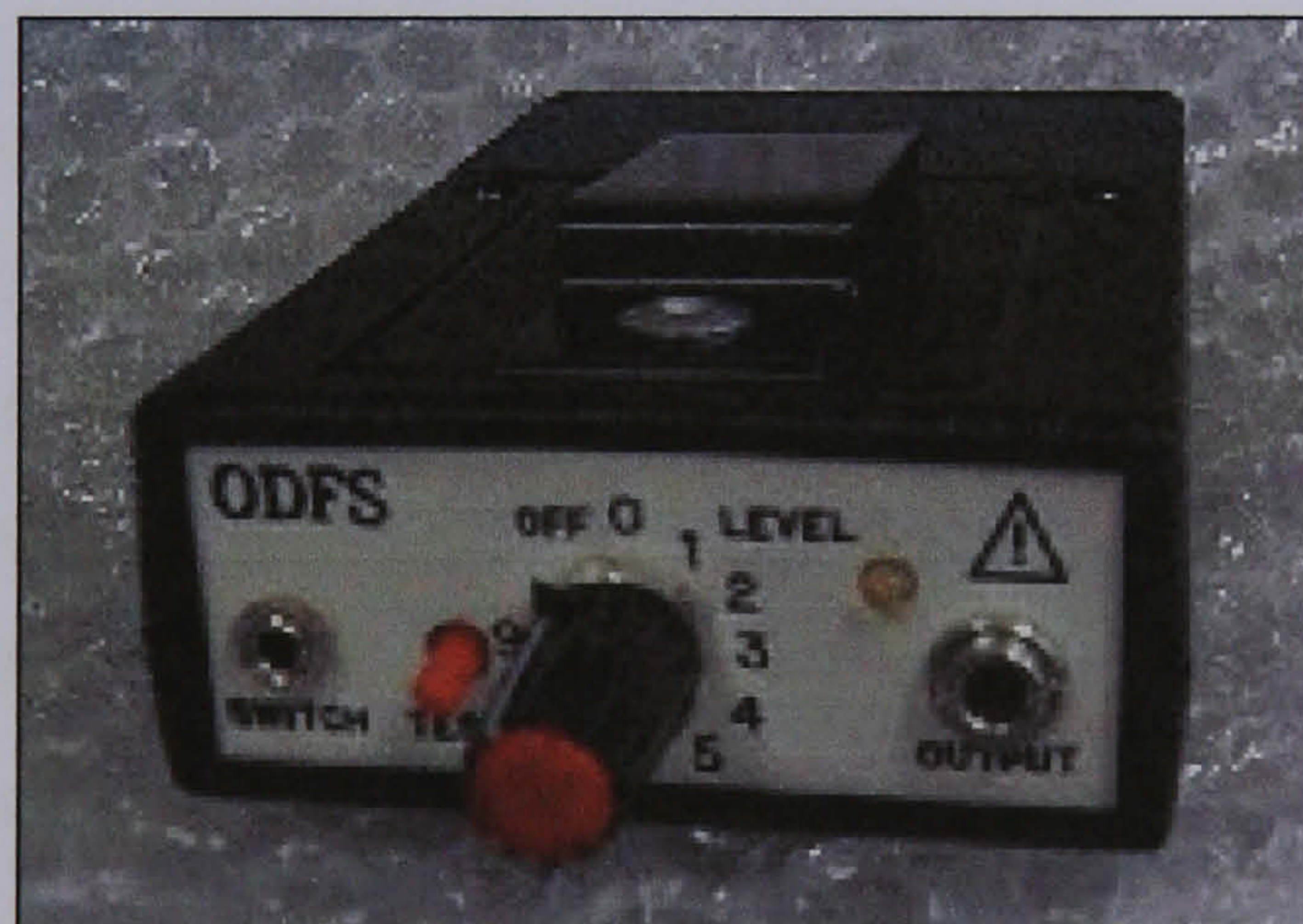
Figure 6-18: ODFS single channel foot drop stimulator (Salisbury District Hospital, UK)
