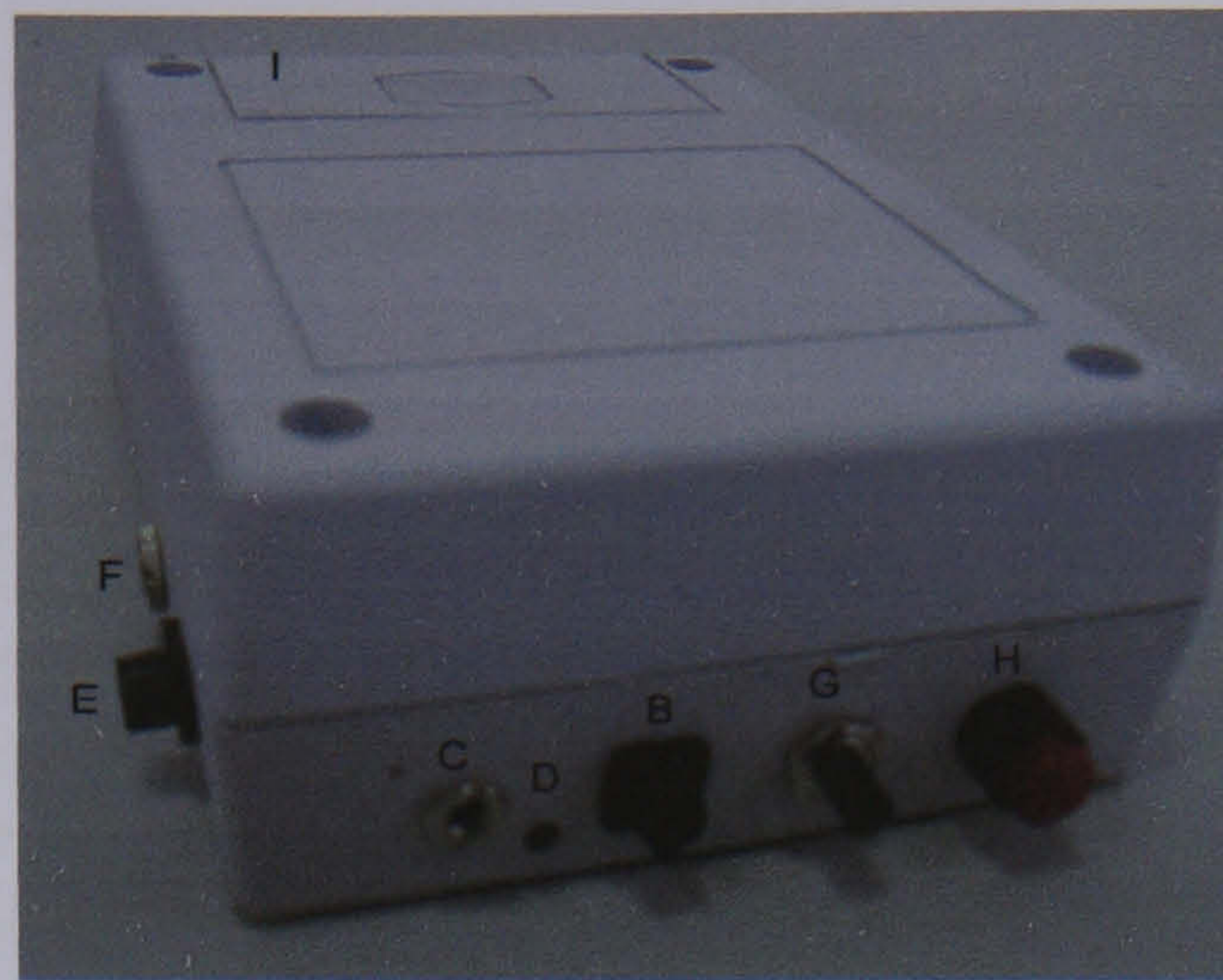
Figure 6-8: The microcontroller-based unit with labelled buttons and connectors (dimensions are 108, 79, 35 mm).
