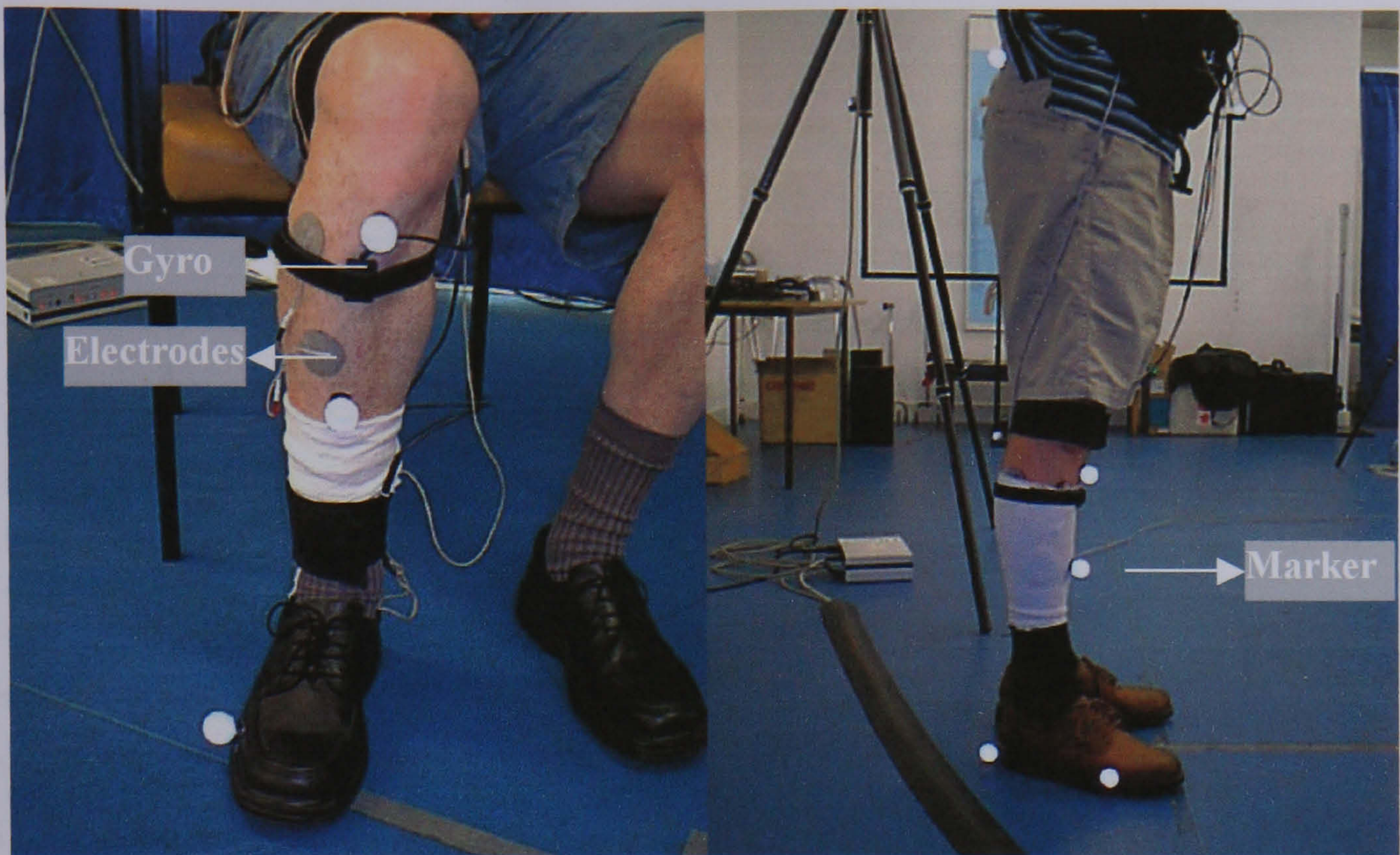
Figure 6-19: Two of the subjects who took part in the study (surface electrodes, Gyro, markers and connecting wires in these frontal and side views).
